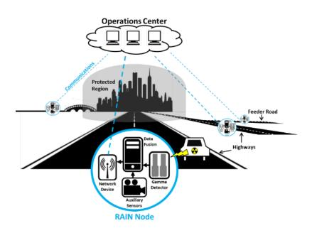
Vehicle scanning at highway speeds to provide actionable information to law enforcement – fused radiation detectors, cameras, and license plate readers.
